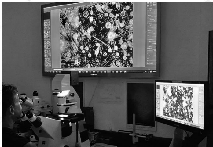
microscopic analysis of phytoplankton in the CMB lab (Utermöhl sedimentation method)
