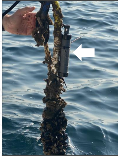
submersible data logger affixed to leader above fuzzy rope
