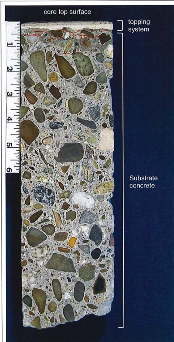
Fig. 11 Lapped, cross-sectional concrete surface of Core 16. The core consists of a topping system and substrate concrete. Some horizontal microcracks (highlighted red) are present in the top 0.9 in. of the substrate concrete. These microcracks may or may not be ASR-related.
