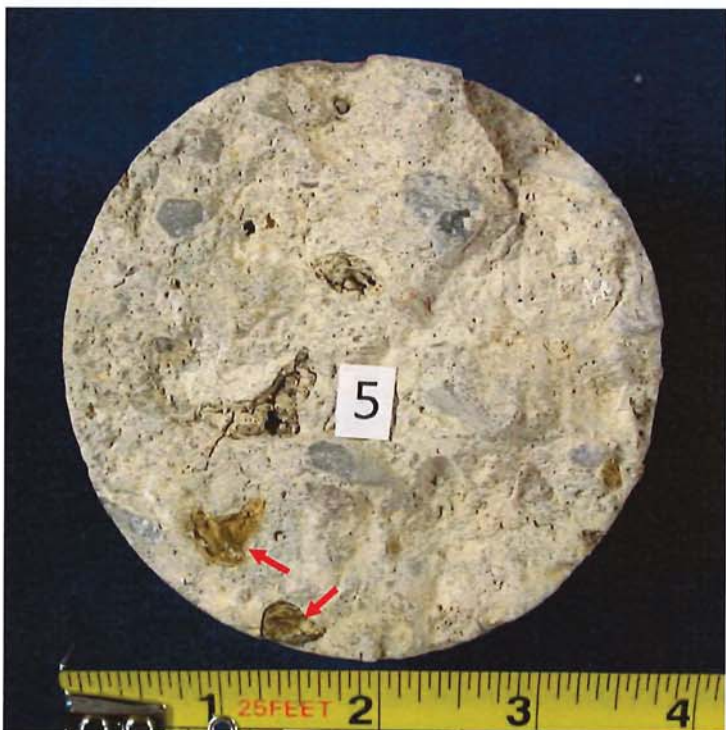
Fig. 5.2 Two of the as-received fractured surfaces of Core 5, illustrating evidence of ASR within the concrete.
