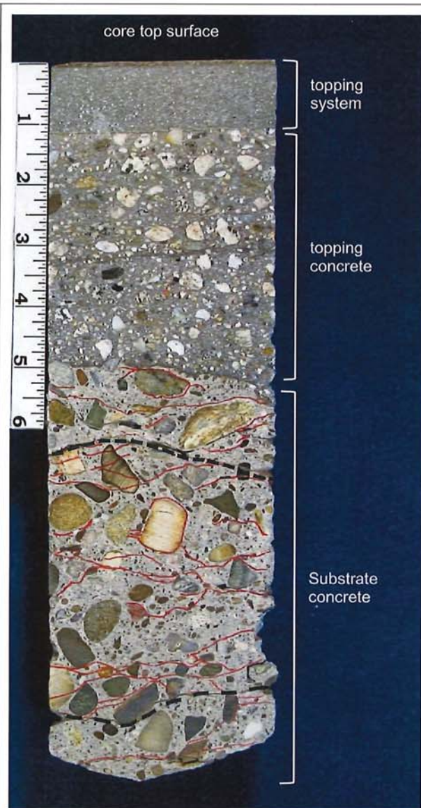
Fig. 4 Lapped, cross-sectional concrete surface of Core 6. From top to bottom, core consists of a topping system, topping concrete, and substrate concrete. Core was received fractured horizontally into 3 segments within the substrate concrete; dashed-black lines depict the fractures. Microcracks (highlighted red) within the substrate concrete are substantial and are assessed to be ASR cracking. fractured through end of core; cause for this crack is not discerned petrographically.
