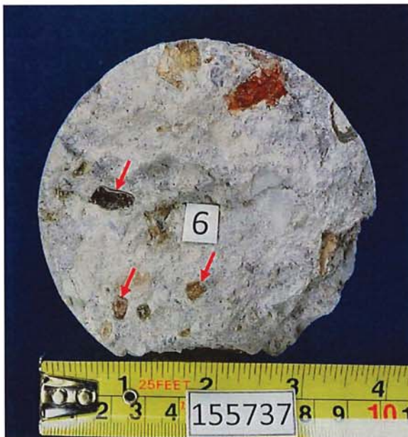
6.1.b. Core side surface. Several reacted aggregate particles (red arrows) are present.
