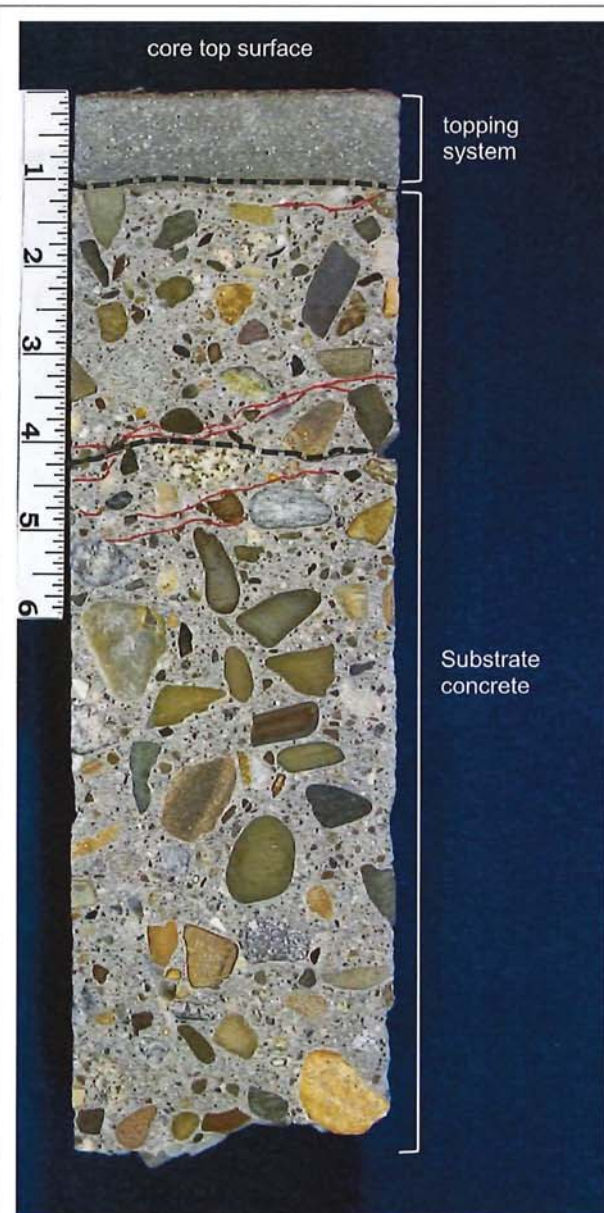
Fig. 10. Lapped, cross-sectional concrete surface of Core 13. The core consists of a topping system and substrate concrete. Core was received fractured horizontally into 3 segments; dashed-black lines depict the fractures. Several horizontal (at slight angle) microcracks occur near the full fracture crack, several above and several below within a substrate concrete depth interval of 2.2 to 4 in. Another horizontal microcrack is present in the top 0.3 in. of the substrate concrete. These microcracks may or may not be ASR-related.
