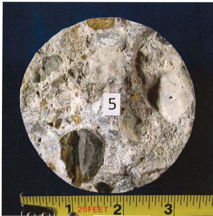
5.2.a. The surface is coated with white secondary deposits of ettringite and ASR gel.
