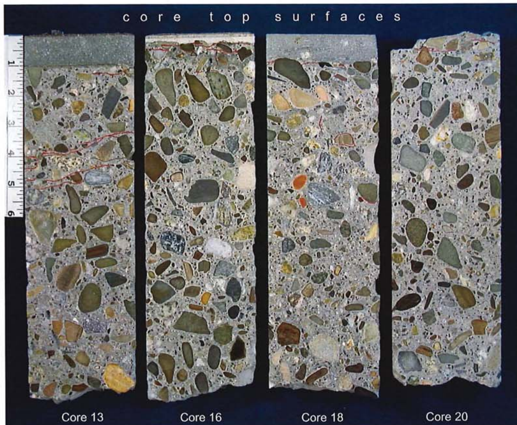
Fig. 2 Side by side comparison of lapped, cross-sectional (longitudinal) concrete surfaces of Cores 13, 16, 18, and 20. Cores 13, 16, and 18 have a topping system. The remainder of the cores consists of substrate concrete (tan paste concrete), which contains similar aggregate types among the 4 cores. The coarse aggregate is a natural gravel composed of a wide variety of similar rock types. The fine aggregate is a natural sand composed mainly of quartz and quartzite, with lesser amounts of similar rock types.
