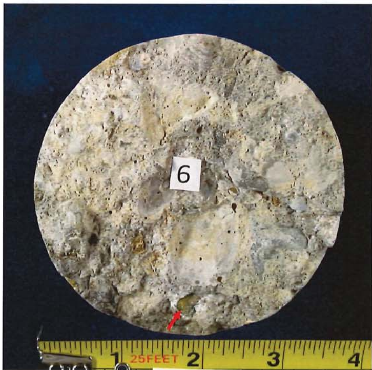
Fig. 6.2 Two of the as-received fractured surfaces of Core 6, illustrating evidence of ASR within the concrete.
